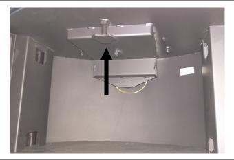
D17 - unscrew security screw to loosen the rotation lock
